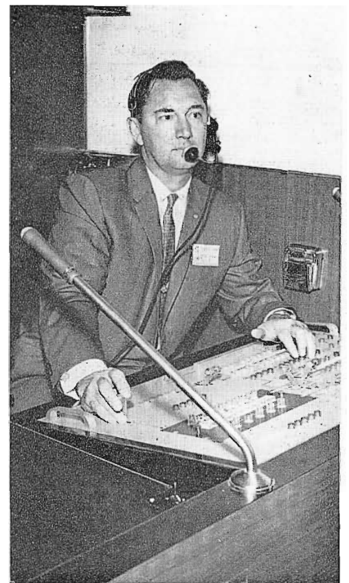
FIG. 6. Mr. Charles Schmidt, video engineer, Skelton Studios, at production control desk. This transistorized switching system and effects control panel was custom designed. It handles 10 inputs from color and monochrome cameras, slide and film projectors, and tv tape machines. The system affords a choice of more than 150 RCA special effects.
